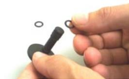
**NOTE:** The 'O' Rings must locate in the grooves shown below, and not the circlip groove nearest the end.
