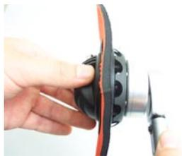
**☞ NOTE:** Rotate the valve body (5) clockwise until it reaches its stop and, whilst holding the valve, rotate the back nut (11) to tighten. This aids assembly and also reduces the chance of damaging the backing patch or suit. An Apeks backing patch (AP0166) should be used to ensure no leaks can occur between the valve and the suit.
