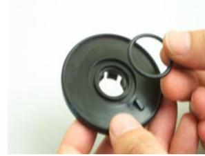
3. Slide two new, lubricated 'O' Rings (3) onto the stem of the button (2) and locate in the two grooves.
