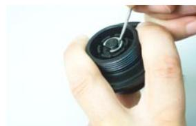
4. Lift out the button (2) and spring (4) from the valve body (5).
