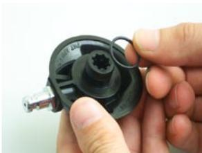
2. Place a new, lubricated 'O' Ring (6) into the groove of the base (9).
