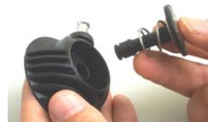
5. Push button (2) into valve body (5), and whilst fully depressed, push the circlip (8) into the groove of the button.
