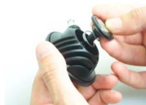
5. Screw the separation tool (AT7009) onto the thread of the valve body (5) until the base (9) and valve body separate. Once complete, unscrew the separation tool from the valve body.
