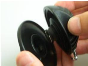
7. Rotate the valve body (5). It should rotate smoothly through an angle of approximately 350° without being over tight.
